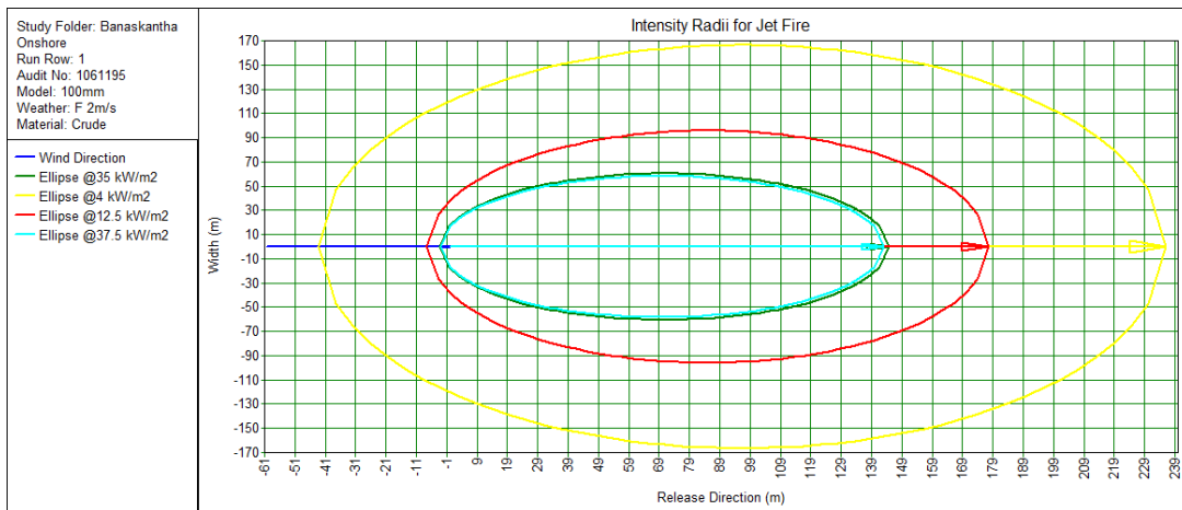
INTENSITY RADII FOR JET FIRE DUE TO 100 MM LEAK OF CRUDE IN IS 02
