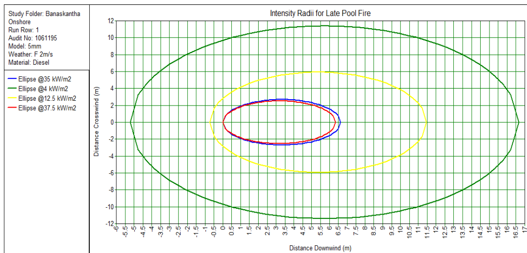
INTENSITY RADII FOR LATE POOL FIRE DUE TO 5MM LEAK OF DIESEL IN IS 07
