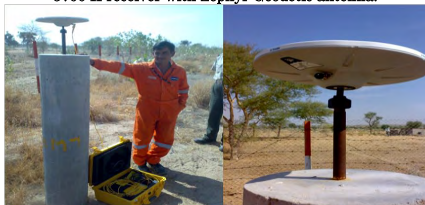
Figure 5: Campaign station showing pillar fitted with rover Trimble 5700 II receiver and Zephyr Geodetic antenna.
